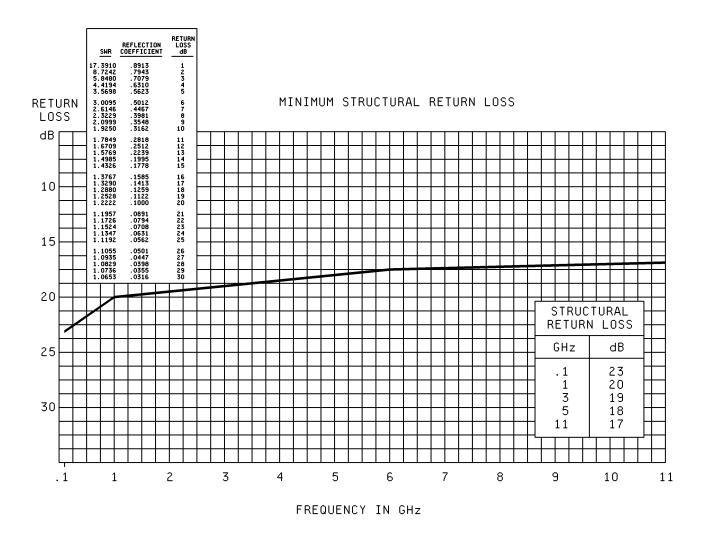
FIGURE 3. Structural return loss.
