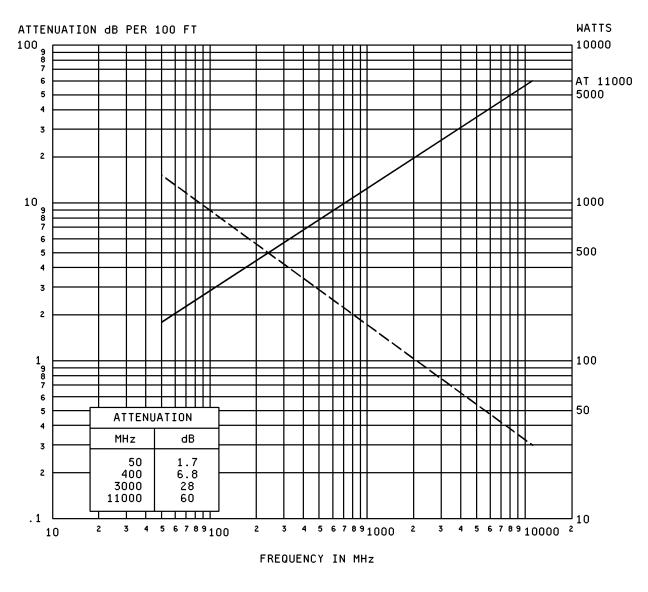
FIGURE 2. Power rating and attenuation.
