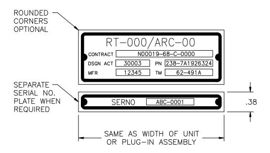
FIGURE 1. <u>Unit plug-in assembly identification plate</u>.
