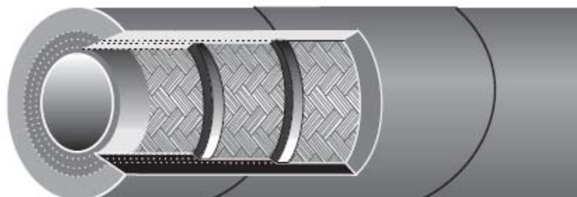
FIGURE 3. MIL-DTL-13531, type III, class A.
