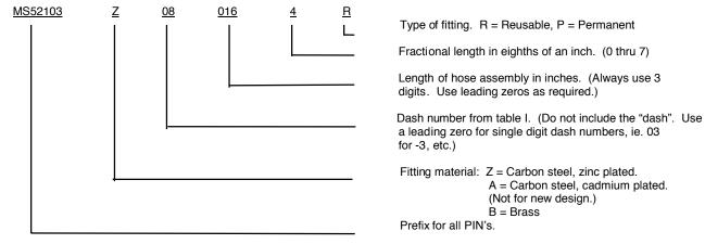
The old MS number is used in the PIN to maintain backwards compatibility with existing parts and higher level drawings. Some existing MS PIN's do not completely fit the above layout, but they should continue to be used without change.
