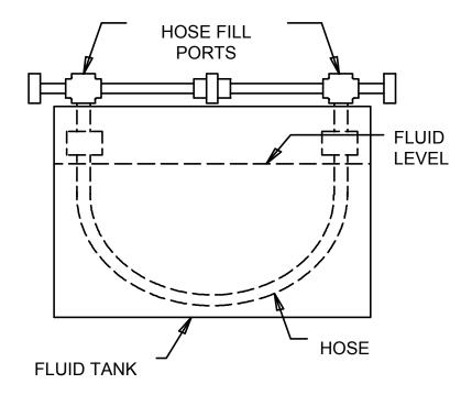
FIGURE 1. Specimen conditioning fluid tank.
