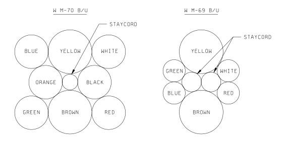
FIGURE 1. Cabling diagrams.
