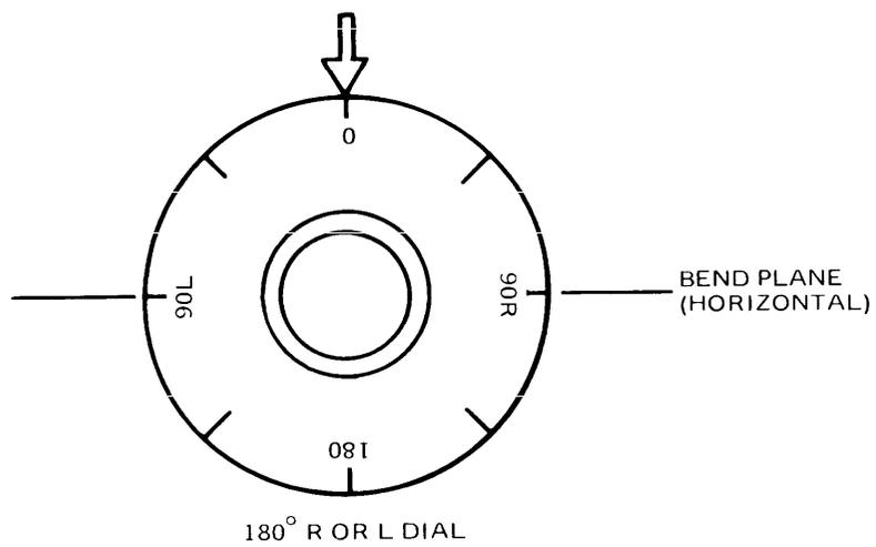
FIGURE 3. TYPES OF DIALS COMMONLY USED WITH TUBE BENDING MACHINES.
