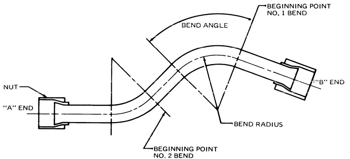
FIGURE 2. TUBE LAYOUT AND FINISHED ASSEMBLY.
