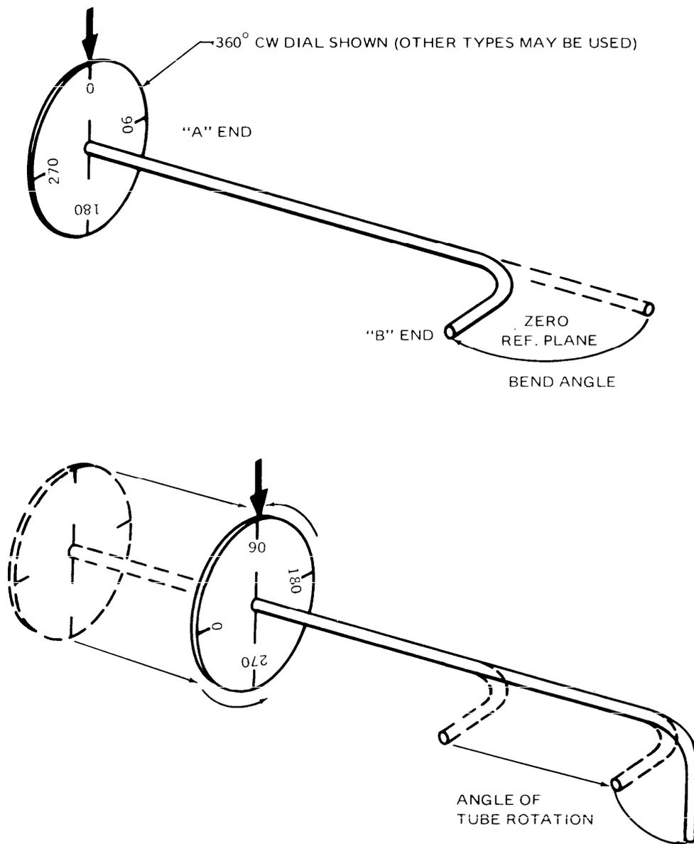
FIGURE 4. ANGLE OF TUBE ROTATION.
