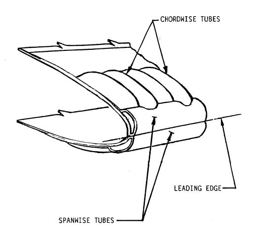
FIGURE 3. Rotorcraft blade pneumatic boot rotary wing aircraft.
