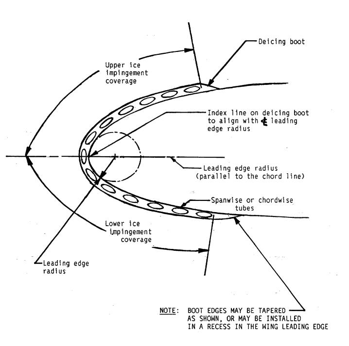
FIGURE 2. <u>Typical deicing boot installation</u> fixed wing aircraft.
