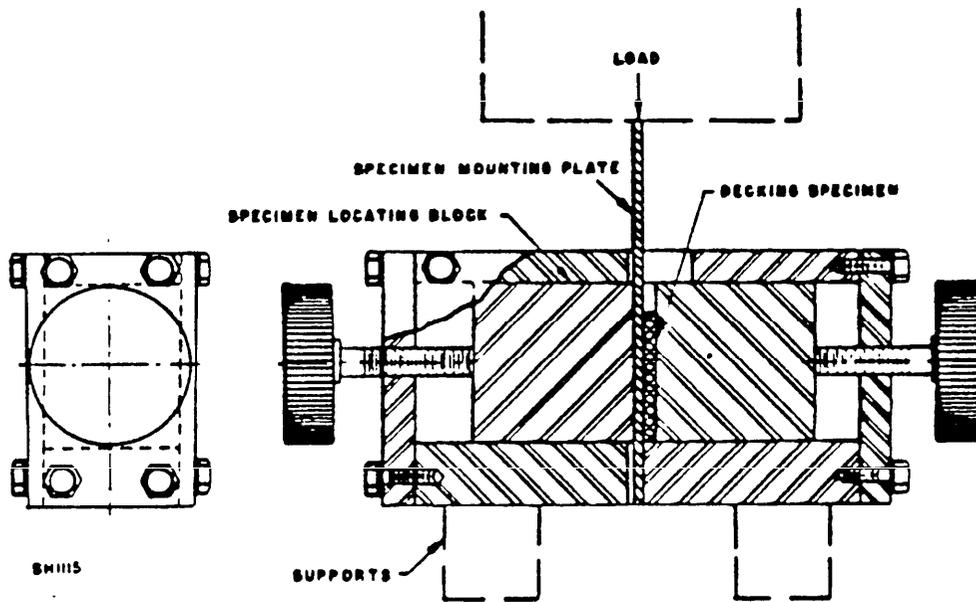
FIGURE 1. Shear test jig for hard-setting deck covering materials.
