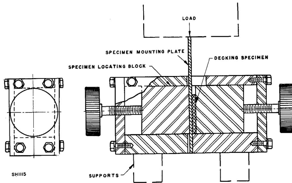
FIGURE 1 - Shear test jig.
