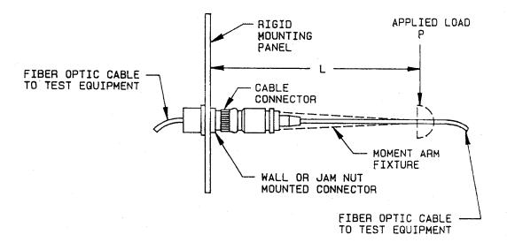
NOTE: Moment arm fixture shall be of a convenient design.
