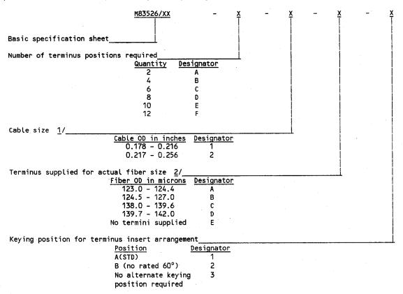
$<sup>\</sup>underline{1}$ / Select cable size and type in accordance with MIL-C-85045.
