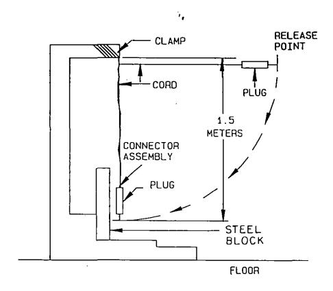
FIGURE 1. Impact test facility.
