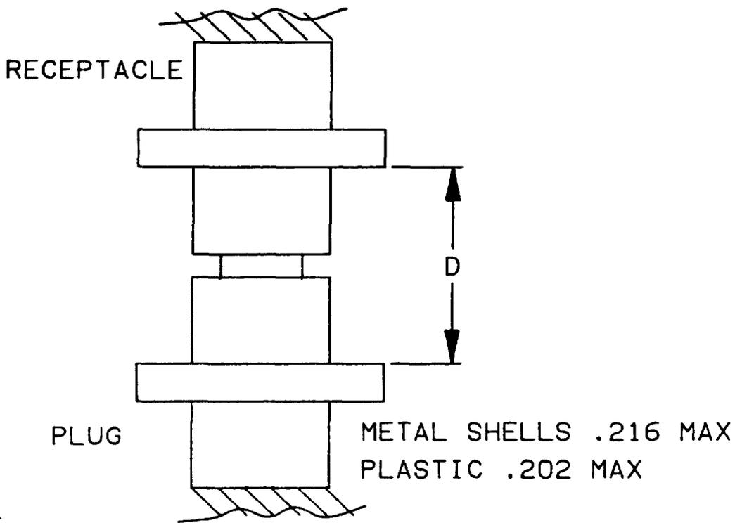
FIGURE 1. Connectors, fully mated.
