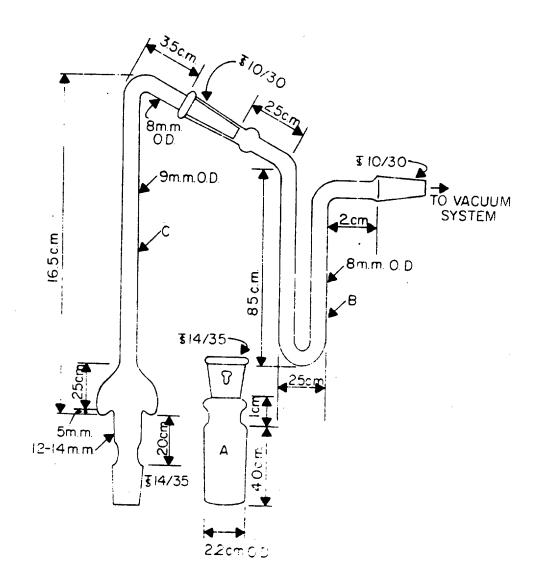
Figure 1. Small-Scale Vacuum Distillation Apparatus
