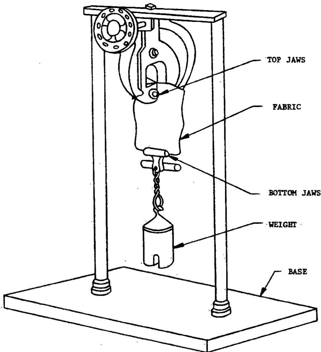
FIGURE 1. Fabric stretch apparatus.
