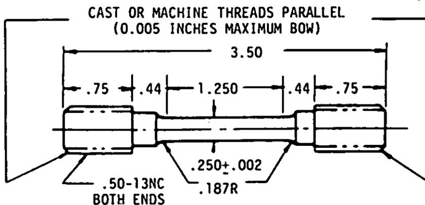
FIGURE 1. Tensile specimen.**4.3 Classification of inspections:**
