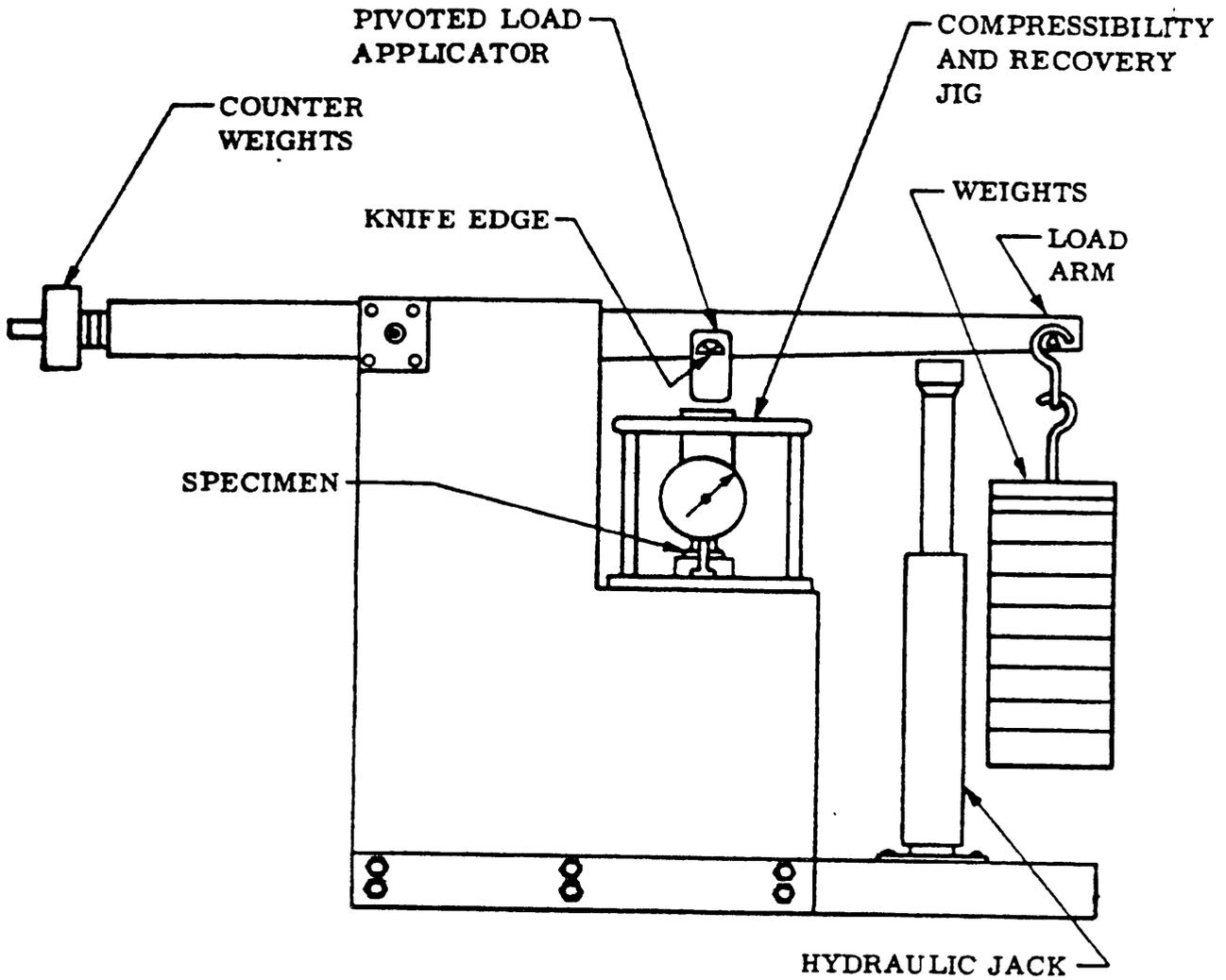
FIGURE 1. Compressibility testing machine.
