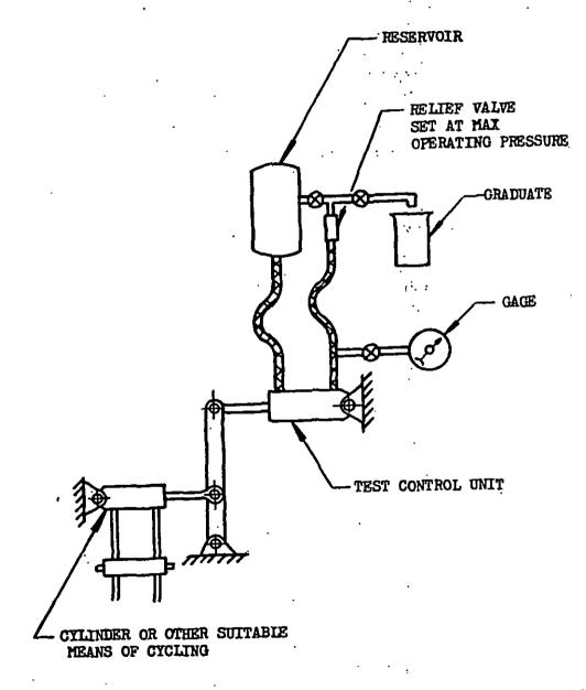
RETURN OF THE TEST CONTROL UNIT MAY BE BY MEANS OF ITS OWN RETURN MECHANISM INSTEAD OF THE CYCLING MECHANISM AS PICTURED.
