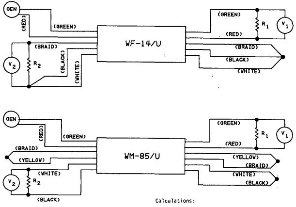
db - dBm reading of  $V_1$  -dBm reading of  $V_2$
