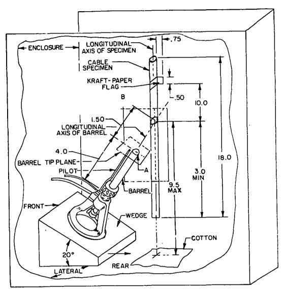
Vertical plane parallel to sides of enclosure and containing longitudinal axis of specimen and longitudinal axis of barrel.
