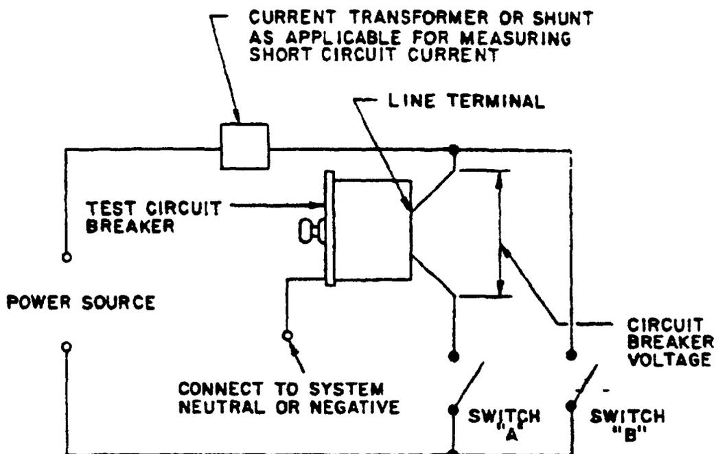
(a) A-C OR D-C SHORT CIRCUIT RUPTURE TEST
