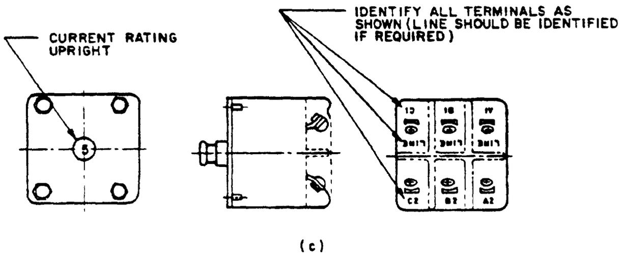
FIGURE 1. Terminal identification.
