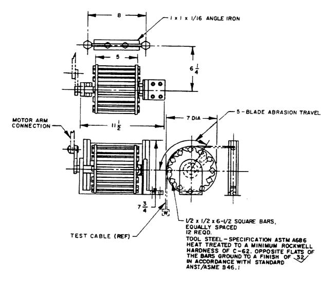
DIMENSIONS IN INCHES. UNLESS OTHERWISE SPECIFIED, TOLERANCES: FRACTIONS= ±1/64
