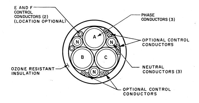
FIGURE 1. Construction of part number M5756/5-001 and -002.
