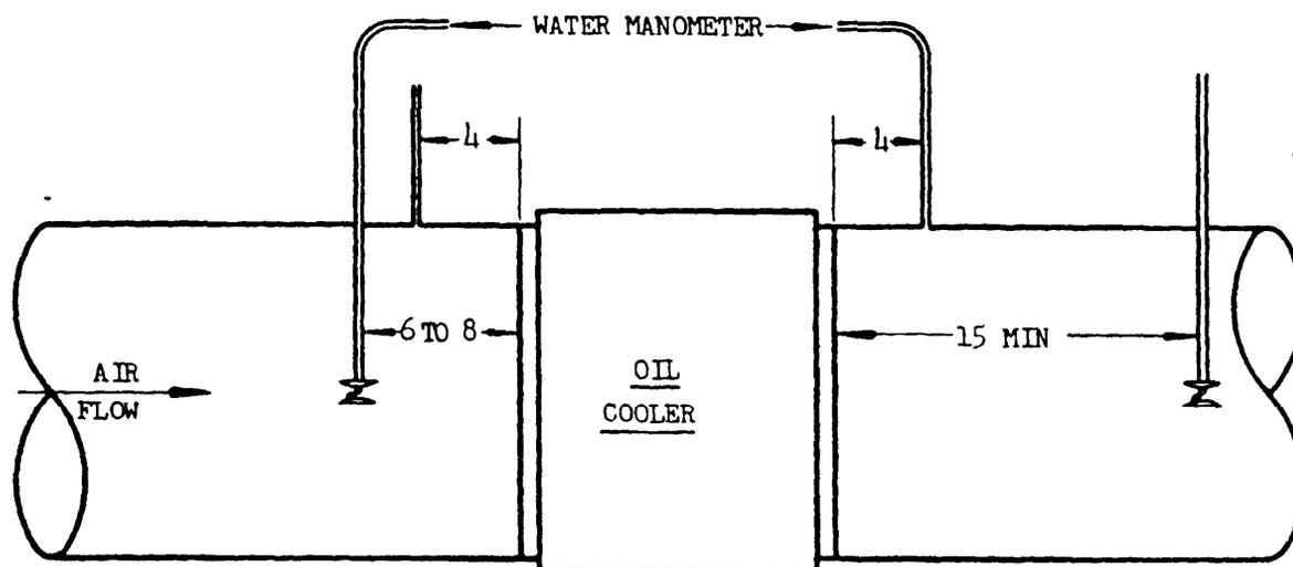
PRESSURE DROP TO BE UPSTREAM TOTAL MINUS DOWNSTREAM STATIC - TOTAL PRESSURES TO BE MEASURED BY SHIELDED TOTAL PRESSURE TUBES OF REVERE INSTRUMENT COMPANY (PART NUMBER R-302-DP) OR EQUIVALENT, LOCATED WITHIN 1 INCH OF THE CENTER OF THE DUCT. DOWNSTREAM TOTAL PRESSURE TUBE IS NOT REQUIRED BUT IS RECOMMENDED AS A MEANS OF CROSS-CHECKING ACCURACY OF THE REQUIRED PRESSURE MEASUREMENTS.
