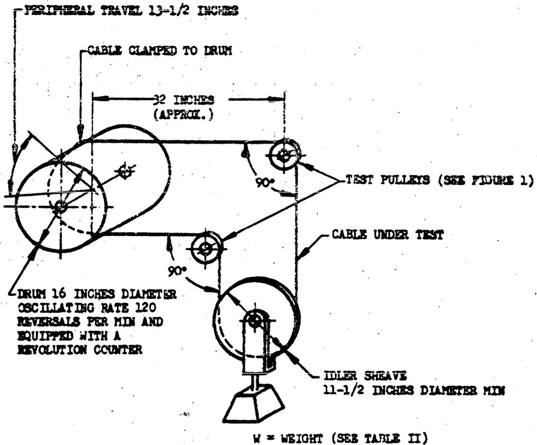
FIGURE 2. Cable Endurance Testing Machine (Diagrammatic).
