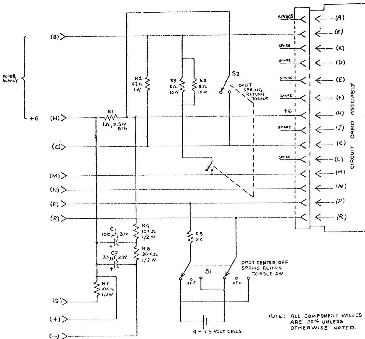
Figure 1. Circuit card tester
