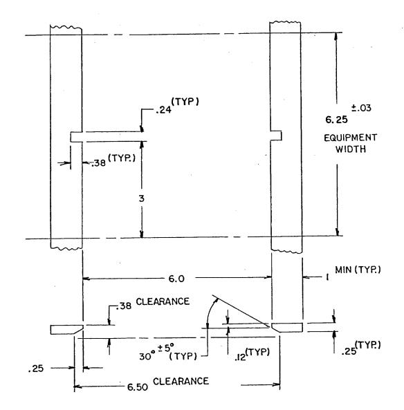
MOUNTING RAILS TO BE SUPPLIED BY AIRFRAME MANUFACTURE.
