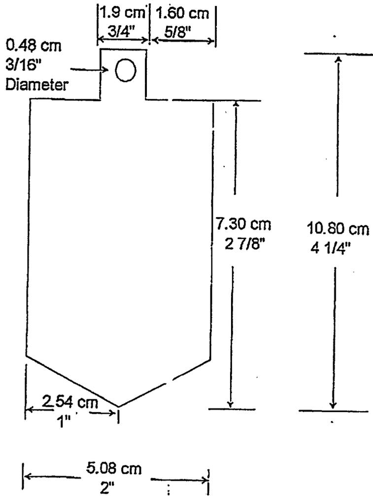
FIGURE 1. Dimensions of stainless steel test panels.
