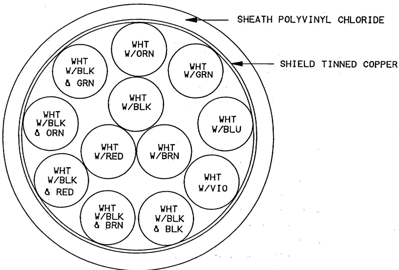
FIGURE 1. Cable configuration.
