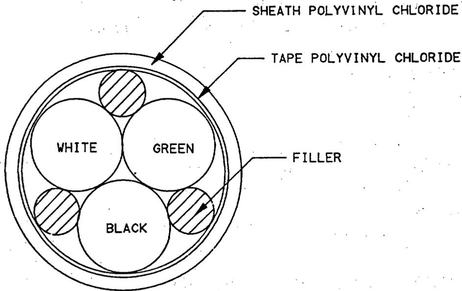
FIGURE 1. Cable configuration.
