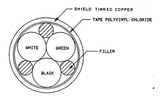
FIGURE 1. Cable configuration.
