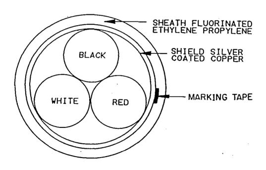
FIGURE 1. Cable configuration.
