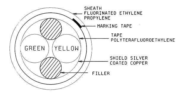
FIGURE 1. Cable configuration.
