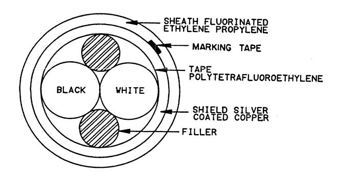
FIGURE 1. Cable configuration.
