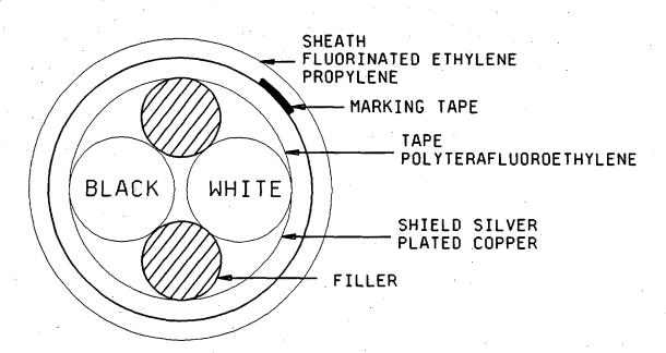
FIGURE 1. Cable configuration.
