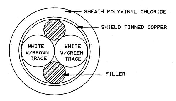
FIGURE 1. Cable configuration.
