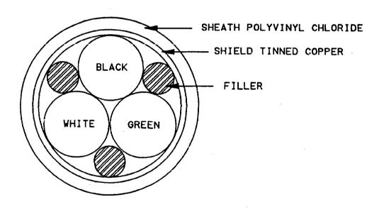
FIGURE 1. Cable configuration.
