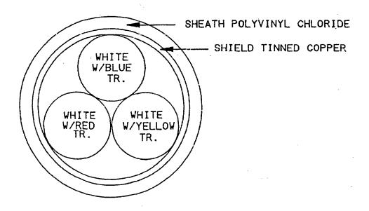
FIGURE 1. Cable configuration.
