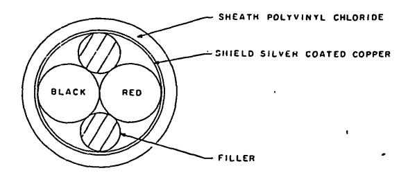
FIGURE 1. Cable configuration.
