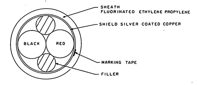
FIGURE 1. Cable configuration.
