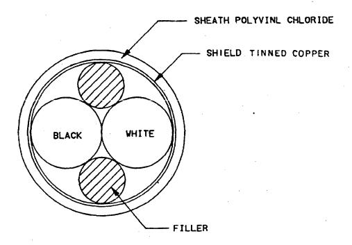
FIGURE 1. Cable configuration.
