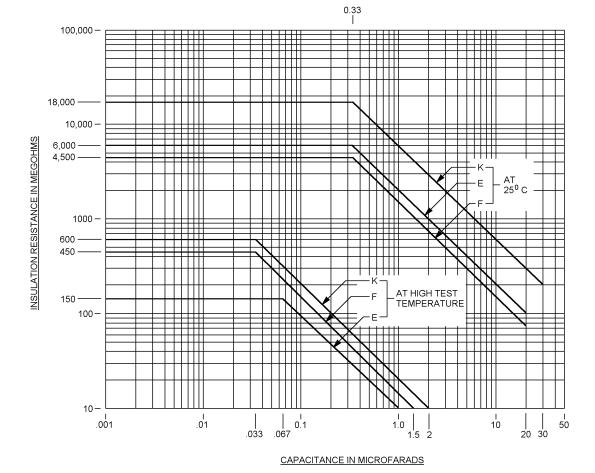
FIGURE 1. Graphical representation of insulation resistance requirements specified in 3.6.1 and table V.
