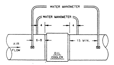
PRESSURE DROP TO BE UPSTREAM STATIC MINUS DOWNSTREAM STATIC. TOTAL PRESSURE TUBES ARE NOT REQUIRED BUT ARE RECOMMENDED AS A MEANS OF CROSS CHECKING ACCURACY OF THE REQUIRED PRESSURE MEASUREMENTS. TOTAL PRESSURES TO BE MEASURED BY SHIELDED TOTAL PRESSURE TUBES OR REVERE INSTRUMENT COMPANY (PART NUMBER R-302-DP) OR EQUIVALENT, LOCATED WITHIN ONE INCH OF THE CENTER OF THE DUCT.
