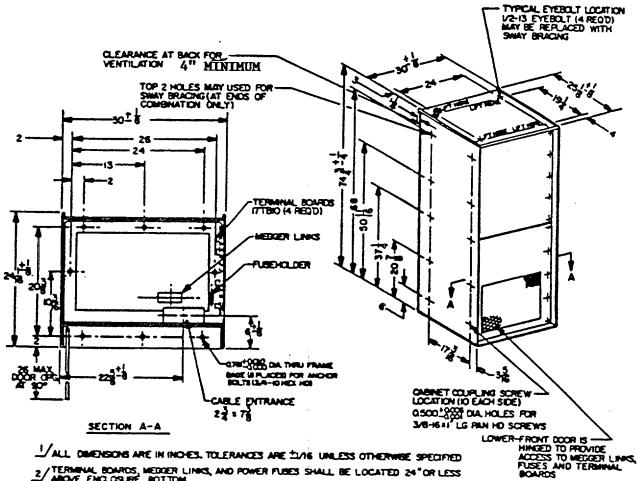
2/ TERMINAL BOARDS, MEDGER LINKS, AND POWER FUSES SHALL BE LOCATED 24" OR LESS
