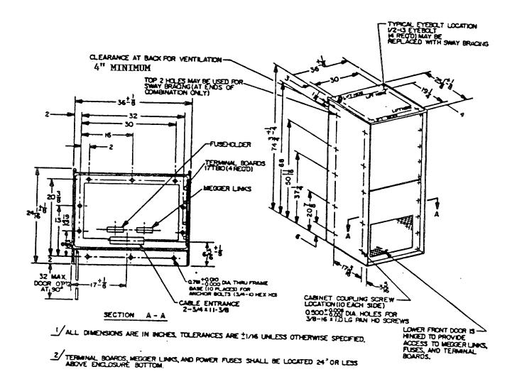
FIGURE 6. 20, 26, 32 and 40 kW power supply, outline drawing.
