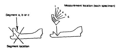
FIGURE 1. Metallographic sectioning.
