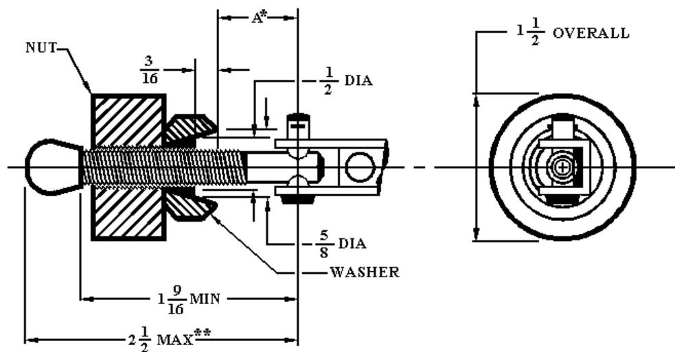
\* CLEARANCE ON OPEN OR EXTENDED POSITION  $1 \frac{3}{8}$  MINIMUM FOR DIMENSION A
