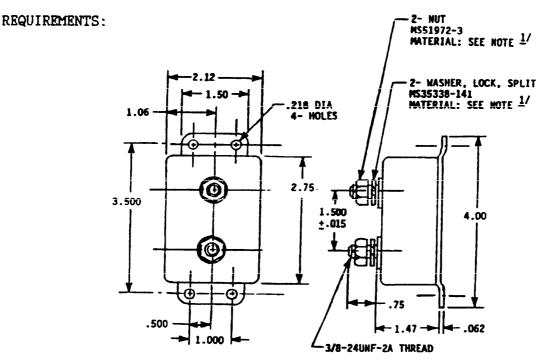
Classification: Type II (Automatic reset), Grade B (Nonwaterproof), Class 2 (over 30 amperes rating).
