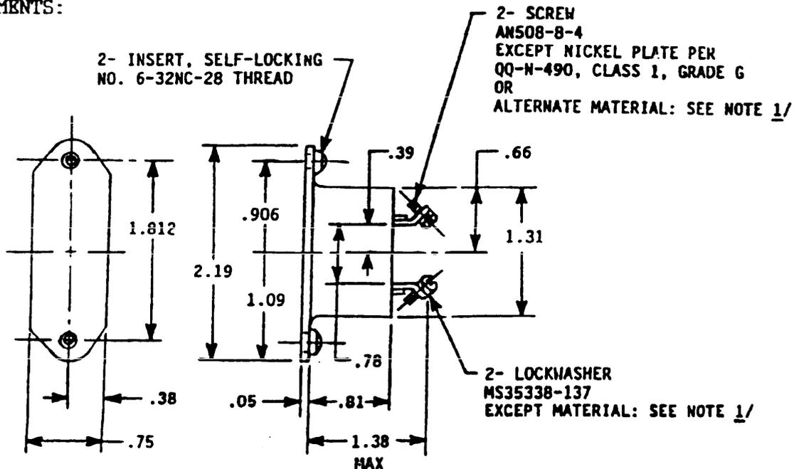
Classification: Type II (Automatic reset), Grade B (Nonwaterproof), Class 1 (over 30 amperes rating). Class 2 (over 30 ampere rating).
