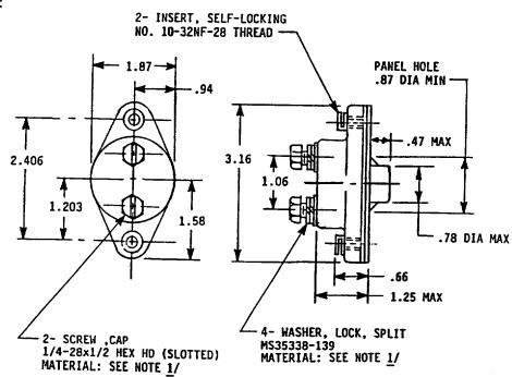
Classification: Type I (Manual reset), Grade B (Nonwaterproof), Class 2 (over 30 ampères rating).
