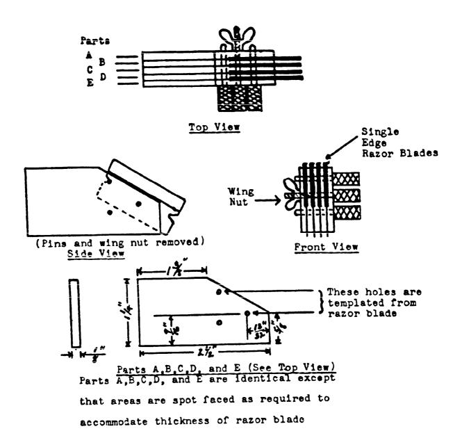
FIBURE 1. Scratching tool used in the low-temperature adhesion test.
