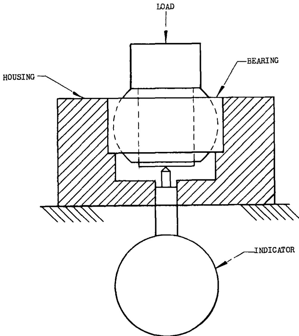
FIGURE 2. Axial test fixture
